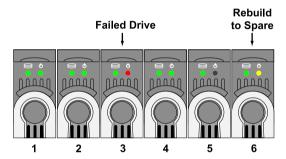
If a physical drive fails in a disk array and there is a spare drive of adequate capacity available, the controller automatically rebuilds the array using the spare drive. In this example, physical drive 3 failed and the array is rebuilt using physical drive 6, the revertible spare drive.
